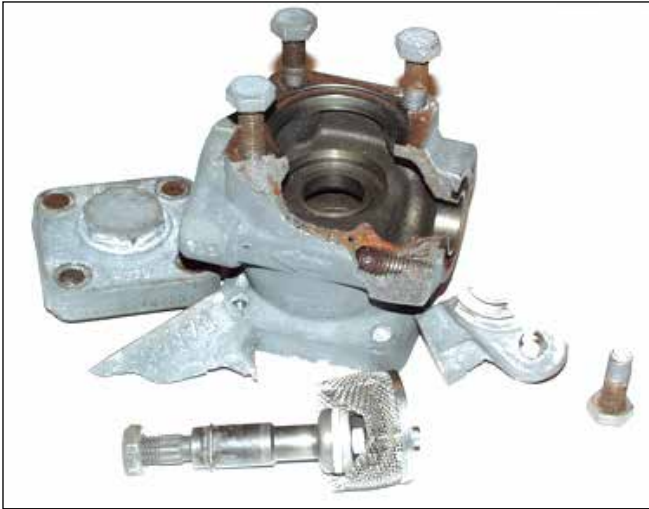
Figure 9: PM valve, incorrectly installed in wet return line
