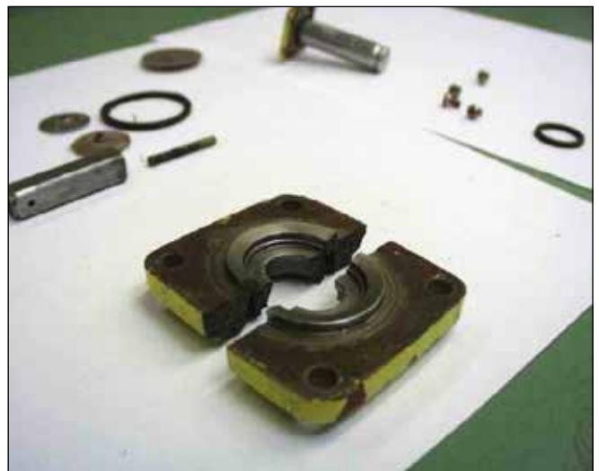
Figure 8: Bottom plate of damaged solenoid valve
