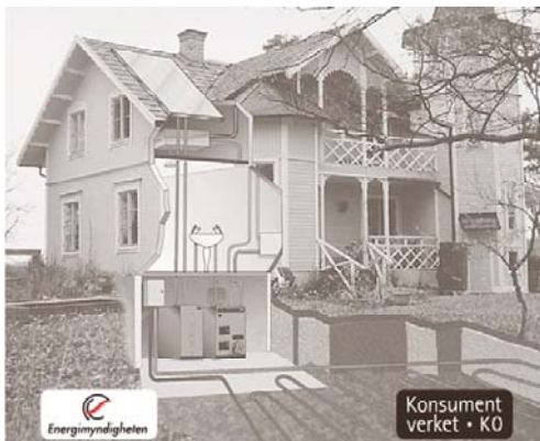
Domestic Heat Pump with shallow ground heat source
