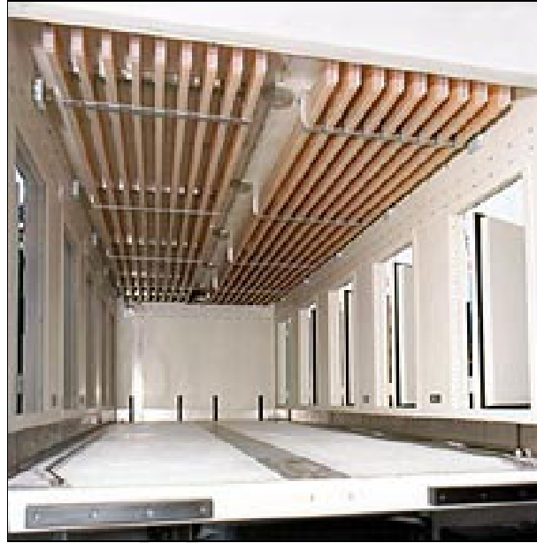
Figure 3. Example of Eutectic Beams (source:Frigoblock, www.frigoblock.de )
